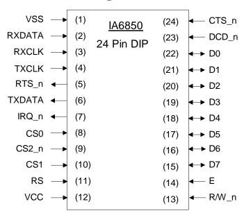
The IA6850 is an ACIA megafunction used to interface a microprocessor to a serial communications channel, and is functionally equivalent to the Motorola MC6850. This function receives and transmits data in a variety of configurations including 7 or 8 bit data words, odd, even, or nor parity, and 1 or 2 stop bits.
