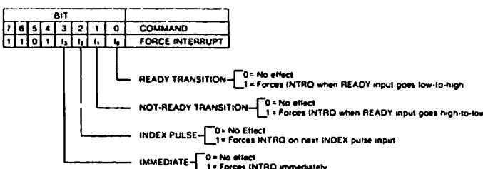
Figure 3. Force Interrupt Command Flags
