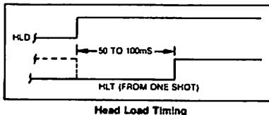
When both HLD and HLT are true, the FDC179X will then read from or write to the media. The 'and' of HLD and HLT appears as a status bit in Type I status.
