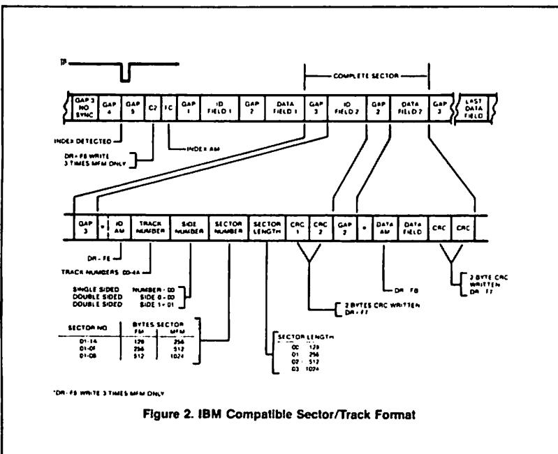
Figure 2. IBM Compatible Sector/Track Format
