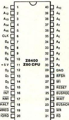
Figure 2a. 40-Pin Dual-In-Line Package (DIP) Pin Assignments
