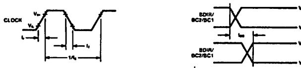
Fig. 7 CLOCK AND BUS SIGNAL TIMING
